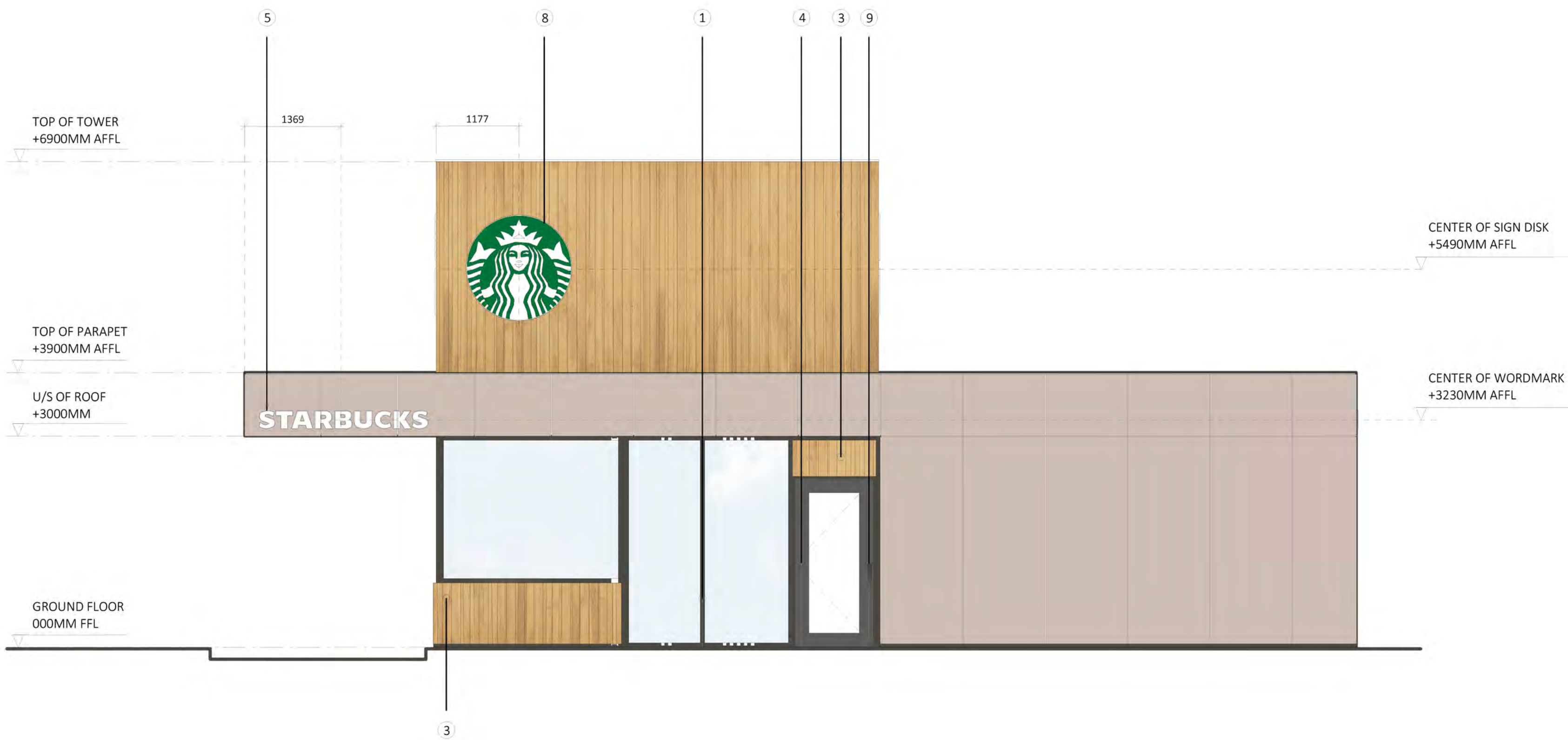
2 EXTERIOR ELEVATION - SECONDARY ENTRANCE 1:100
